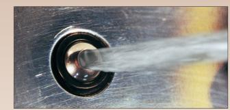
Simply insert the end of allen wrench (included) into the hole in the stainless ball until it engages the hex hole in the acetal body, then tighten the *PlugJet* into the tapped hole until the body is flush.
