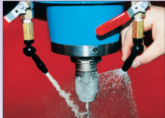
MillJets shown installed on Vertical Machining Center showing wide and narrow spray.
