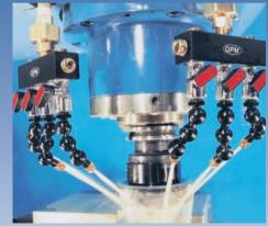
**QPM Manifolds** enable 6 **SwivelMax** nozzles to be used in this face milling operation.
